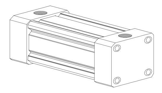
**TYPE:** Repairable, square head, medium bore sizes, double–acting, light to medium duty.
